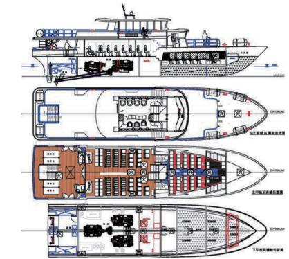
The Froude number of Dapeng Bay No. 6 is 1.2 in the hull linear design. It adopts the Hard Chine ship type and is equipped with 3 MTU 1700 BHP main engines. It reaches 5100 horsepower. The maximum speed can reach 35 knots at full load. it is also equipped with a Impressed Current Anti Fouling system and an independent FM 200 fire extinguishing system, and a 60HP bow thruster improves the equipment quality of general passenger ships.
