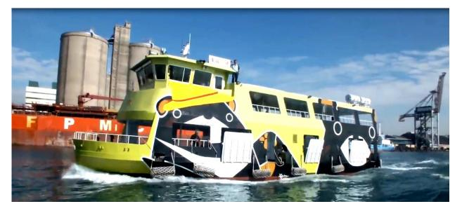
Asia's first electric ferry "CHI FU NO.1" uses lithium battery and solar energy as its main source of power. She was designed by Ship and Ocean Industries R&D center and manufactured by Tinghai Shipbuilding in full accordance with the operational needs of the user, Kaohsiung City Shipping CO. Ltd.
